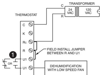
1 Wire the thermostat U1 terminal to the low speed fan for dehumidification control at the equipment as shown. The relay can be set to normally open or normally closed in the installer setup.
