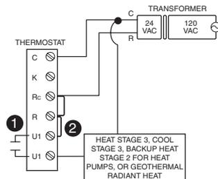
1 U1 terminals are normally open dry contacts when set up for a stage of heating or cooling.
