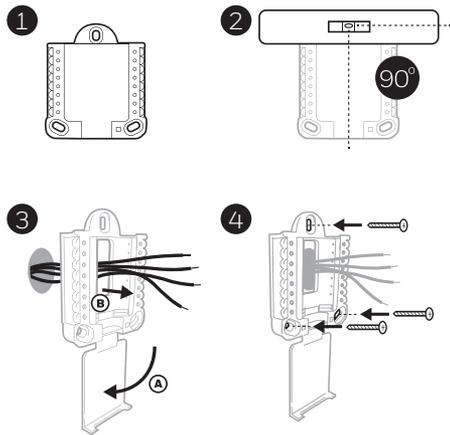
Use 3x supplied screws (#8 1-1/2 for red anchors and #6 1-1/2 for yellow anchors)
