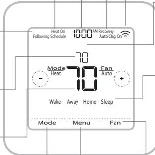
The screen will wake up by pressing the center area of the displayed temperature. If powered by 24 VAC, the screen stays lit for 45 seconds after you complete changes.
