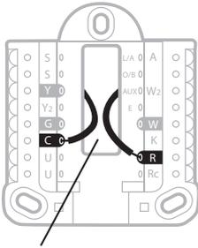
Insert **R** and **C** wires into designated terminals for primary AC power (C terminal is optional if batteries are installed, but it is recommended). Remove wires by depressing the terminal tabs.
