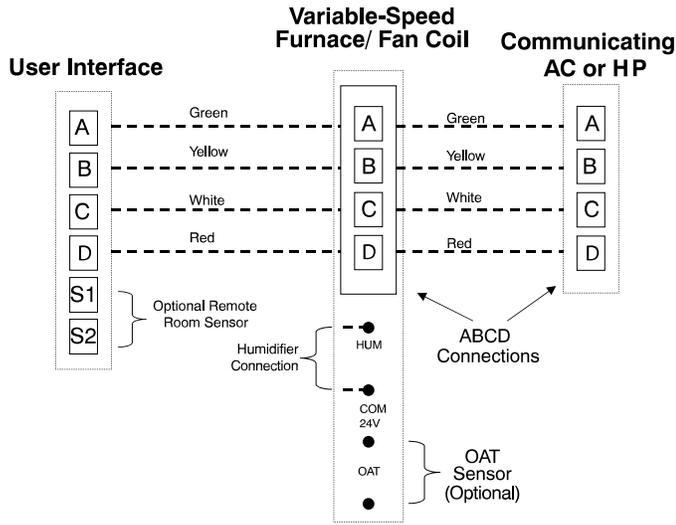
Fig. 1 – Four-Wire Connection Diagram
