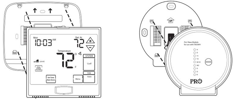
Align the 4 tabs on the subbase with corresponding slots on the back of the thermostat/base module, then push gently until it snaps in place.
