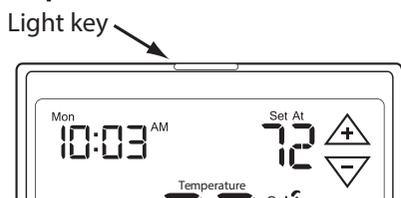
**Important:** DO NOT hold the light button on the thermostat for more than 10 seconds after step 2 above has been completed. Holding the light button down will break the communication link and the base module button will need to be pressed again to reestablish communication.
