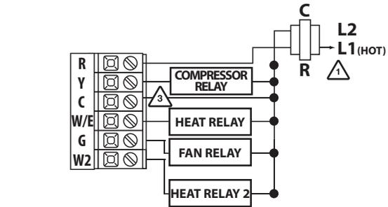
**Note:** This thermostat is only compatible with ONE transformer systems.
