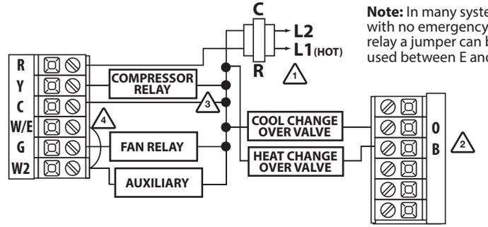
**Note:** In many systems with no emergency heat relay a jumper can be used between E and W2.
