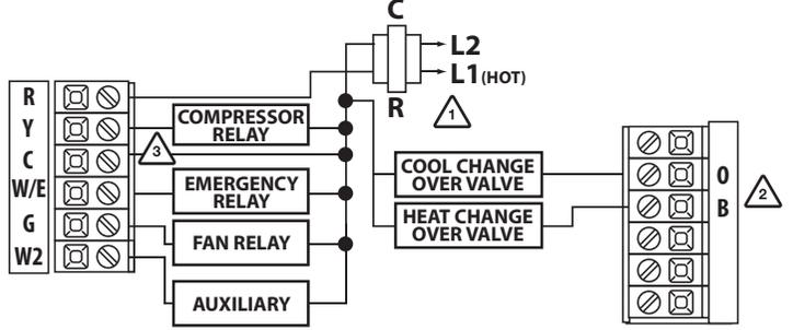
**Conventional System 1H/1C, 2H/1C (Heat pump set to "OFF" in tech settings)**
