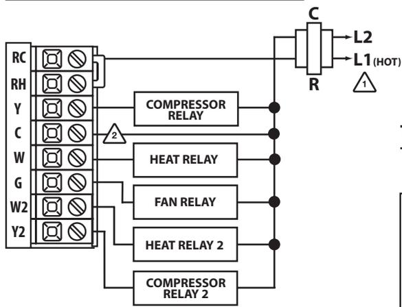
**Note:** This thermostat is hardwire powered when the 24V transformer is connected to the Common and RC terminals of the thermostat.
