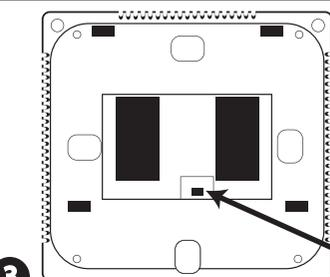
**Gas:** For systems that control the fan during a call for heat, put the fan operation switch to the GAS position.
