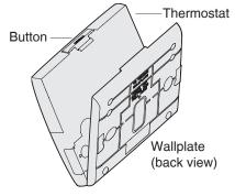
2 Mount wallplate as shown. Mount new wallplate using screws and anchors included with the thermostat.
