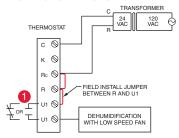
Wire the thermostat universal relay to the low speed fan for dehumidification control at the equipment. The thermostat relay can be set to normally open or normally closed in the thermostat installer setup.
