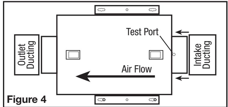
2. Ensure duct joints and exterior penetrations are sealed with caulk or other similar material to create an air-tight path to minimize building heat loss or gain and to reduce the potential for condensation. Place/wrap insulation around duct and/or fan in order to minimize possible condensation buildup within the duct, as well as building heat loss or gain.
