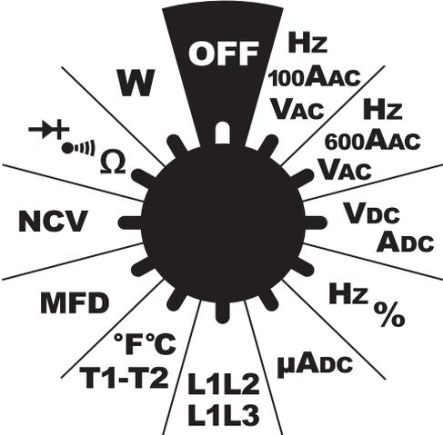
The SC680 is loaded with the measurement parameters essential for HVACR professionals. Select the parameter on the dial you want to measure with the rotating selector switch.
