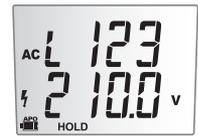
Simply swap any two lines to change the direction. You can verify this by performing the test again.
