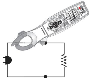
Amps AC (AAC), Frequency (Hz) through the clamp and Inrush AAC current is measured in the VAC/100AAC/Hz or VAC/600AAC/Hz switch position shown above.
