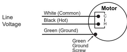
115 VAC Connection, One Speed Motor (Figure 3).
