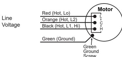
230 VAC Connection, Two Speed Motor (Figure 6).
