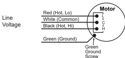
115 VAC Connection, Two Speed Motor (Figure 4).
