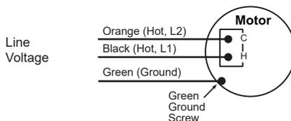
230 VAC Connection, One Speed Motor (Figure 5).
