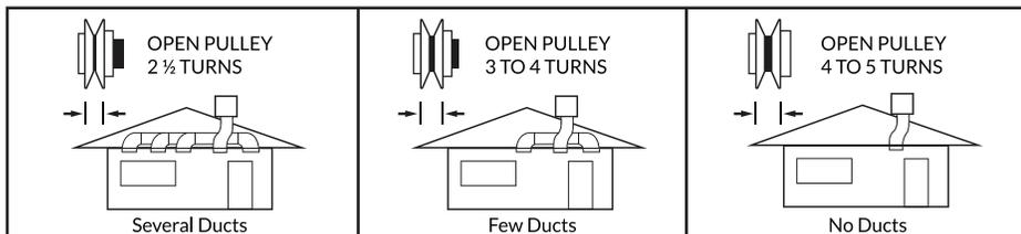
Set Pulley for Air Flow Resistance (Figure 7).
