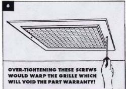
Use ½" grille mounting screws and predrilled holes to mount the ceiling grille into position on the vent.
