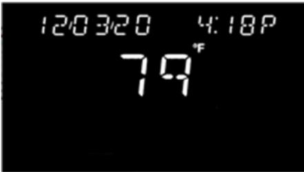
The banner scrolls through date and time, humidity, outdoor air temperature, if configured, and any active faults or system events. The room temperature is prominently displayed.
