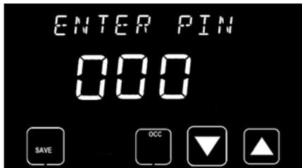
This screen has an **OCC/UNOCC** button to temporarily override the program schedule settings without knowing the PIN. The PIN must be entered for all other thermostat changes. Pressing the **OCC/UNOCC** button temporarily overrides the program schedule settings with the occupied or unoccupied settings. This override remains active until the next time range in the program schedule or until the **MAX HOLD** time expires.
