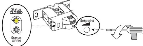
2. Slowly turn the setpoint screw clockwise until the Status Open LED just turns on.
