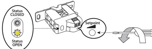
3. Turn the setpoint screw an additional 1/4 turn clockwise for operational margin.
