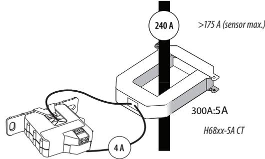
**DANGER:** 5A CTs can present hazardous voltages. Install CTs in accordance with manufacturer's instructions. Terminate the CT secondary before applying current.
