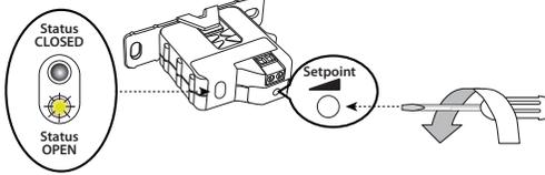
2. Slowly turn the screw counter clockwise until the Status Closed LED turns on.
