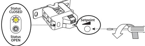
3. Turn the screw an additional 1/4 turn counter clockwise for operational margin.
