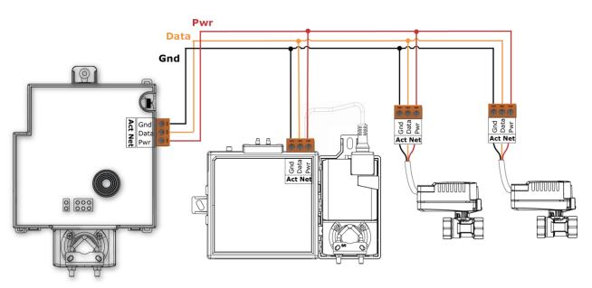
The TV-VAVB3-E2 supports Act Net communication to the Act Net devices on a bus with a maximum length of 300 feet (91.44 meters). The bus should be wired with copper conductors of an appropriate size (18 AWG or larger) to compensate for voltage drop and ensure that bus voltage does not drop below 19.2 Vac or 21.6 Vdc.
