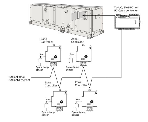
The following illustration shows the TV-VAVB3-E2 in a typical i-Vu® Control System.
