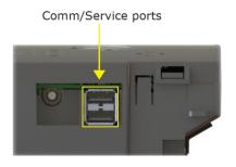
**CAUTION** The USB local access cable provides a common ground connection between the computer and the controller it connects to. Damage to the controller and possibly the computer's USB port will occur if the controller's input power polarity was not maintained and was also not properly grounded (floating). If you are not sure of the wiring polarity and that the controller was properly grounded, use a USB isolator between the computer and the controller.
