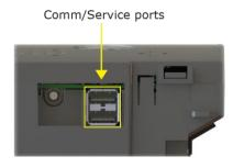
To access the controller setup pages and use the **Local Network** tab, you must first connect to and manually address one TV-VAVB3-E2. For instructions on connecting, see *Addressing the TV-VAVB3-E2 through the Comm/Service ports* (page 16). Navigate to http://local.access or http://169.254.1.1 to access the pages. Then set up the address on your selected TV-VAVB3-E2 on the **Ports** *tab* (page 89).
