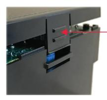
Press tab and pull up to open and remove cover
