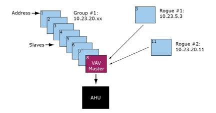
**EXAMPLE #3**: The above network plus sub-masters and their slaves. (For VAV systems only. VVT systems do not support sub-masters.) The sub-masters exchange data between their slaves and the VAV Master, and the VAV Master handles data exchange for the whole system including the Air Source.
