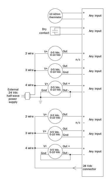
4 Connect binary and analog output wiring to the screw terminals on the TV-VAVB3-E2 and to the controlled device.
