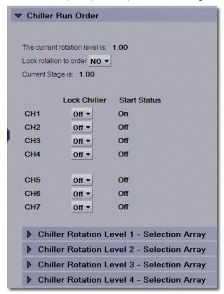
**NOTE** Currently, the Dissimilar-Sized Chiller Manager is limited to Add/Drop applications with 1 small and 3 large chillers. This requires 7 steps of control, as shown below using 7 machines and 7 steps.
