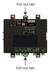
2 Place the controller on the DIN rail so that the rail is in the trough on the back of the controller.
