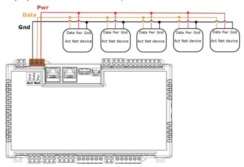
The TV-UC253-V supports Act Net communication to the Act Net devices on a bus with a maximum length of 300 feet (91.44 meters). The bus should be wired with copper conductors of an appropriate size (18 AWG or larger) to compensate for voltage drop and ensure that bus voltage does not drop below 19.2 Vac or 21.6 Vdc.
