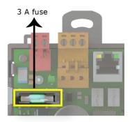
If the TV-UC253-V's power  $\bigcirc$  LED is not lit, this could be due to a blown power fuse.
