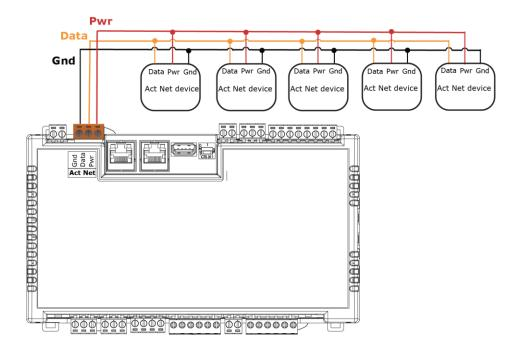
The TV-UCXP683T supports Act Net communication to the Act Net devices on a bus with a maximum length of 300 feet (91.44 meters). The bus should be wired with copper conductors of an appropriate size (18 AWG or larger) to compensate for voltage drop and ensure that bus voltage does not drop below 19.2 Vac or 21.6 Vdc.
