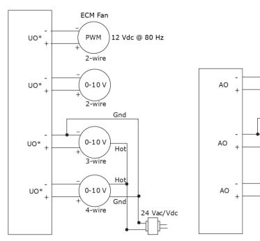
\*Applicable when UO-01 is configured as an analog output.
