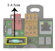
If the TV-UCXP683T's power  $\bigcirc$  LED is not lit, this could be due to a blown power fuse.
