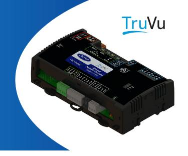
The TruVu™ Advanced Application Controller is ideal for HVAC equipment control, advanced air quality control and most zone-level applications. The TV-UC561 features dual Ethernet ports with built-in fail-safe that supports direct connection or daisy chain topologies using BACnet/IP and 12 points of onboard control. Designed to operate in a wide range of environmental conditions, it is well suited for mechanical rooms, equipment boxes, or almost any other weather-tight location.
