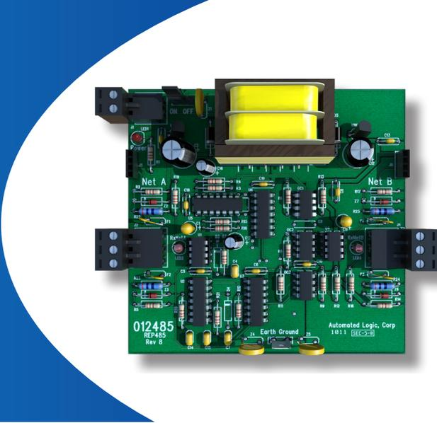
Carrier's ancillary network devices ensure optimum performance for BACnet MS/TP and other EIA-485 networks. These devices install easily and work together to amplify data signals and provide surge protection, bias, and termination to any EIA-485 network.
