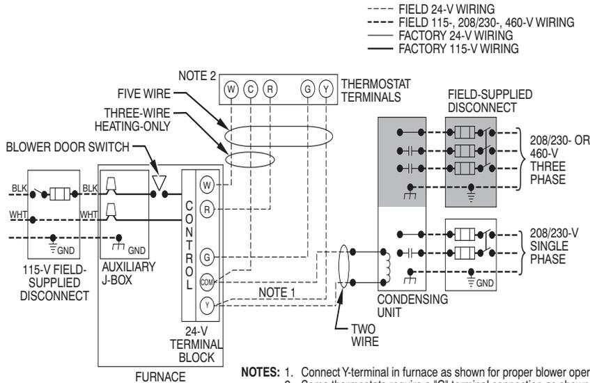
NOTES: 1. Connect Y-terminal in furnace as shown for proper blower operation.
