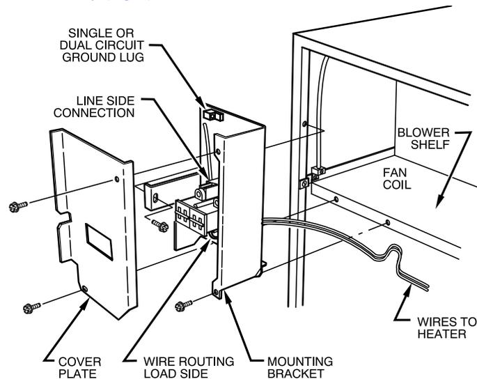
**Fig. 3 – Installation of Circuit Breaker Model Heater**
