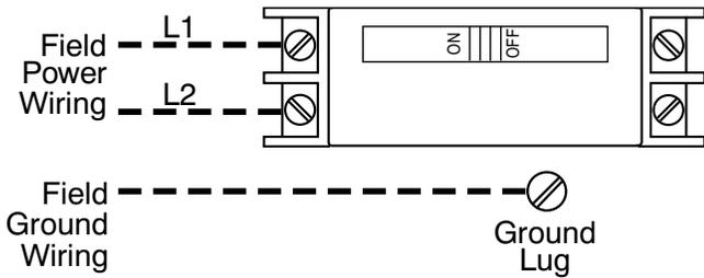
**Fig. 8 – 5, 8 10 kW Circuit Breaker and Disconnect Heaters**
