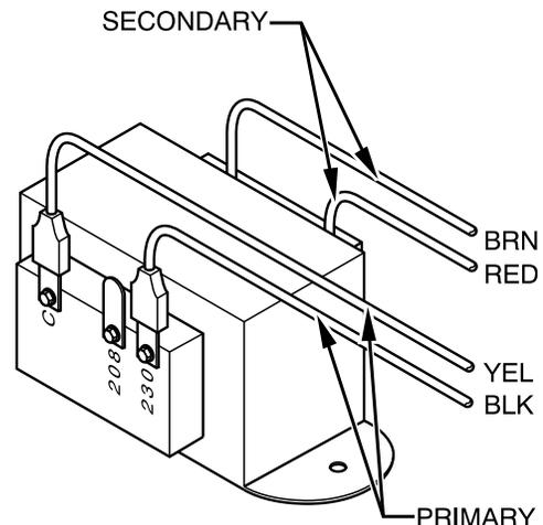
**Fig. 5 – Connection of Transformer**
