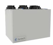
Fantech's VER 100 is an Energy Recovery Ventilator designed for higher static pressure applications. The unit brings a continuous supply of fresh air into a home while exhausting an equal amount of contaminated air. The energy recovery core at the center of the unit transfers heat and moisture from incoming air to the outgoing air that was cooled and dried by the building's air conditioner.
