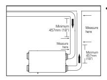
• To avoid airflow turbulence and incorrect readings, the airflow velocity should be measured on a section of steel ducting. Reading should also be taken at a minimum distance of 457 mm (18") from the unit or elbow. Measurement should also be made prior to any transition in the duct work so entire airflow is measured.
