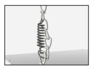
4 Install a spring on each chain. Hook the spring in the links so a loop is created in the chain. The spring will then support the unit's weight and absorb vibrations.
