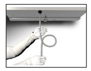
4 Install the drain hose making a "P" trap, secure the condensate line drain connection using the tube clamp provided. Fill the condensate line with water.
