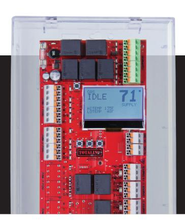
All Totaline TL Series Zone Controllers feature bright, easy to read LCD Displays, LEDs to indicate calls, easy push button setup, screwless terminals, supply air sensors, universal application and a **five-year warranty.**
