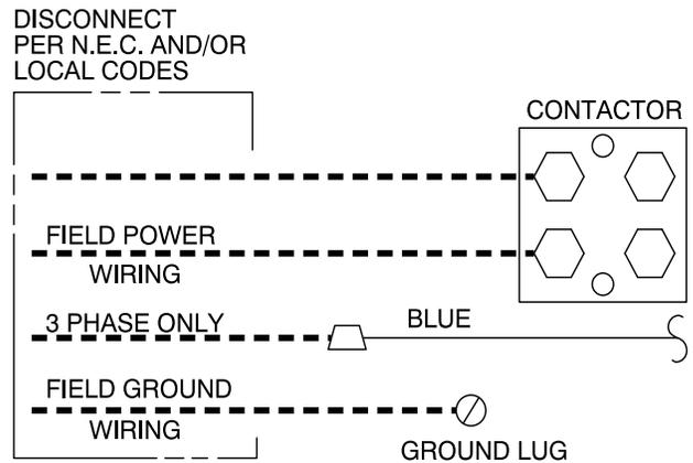
Fig. 8 – Line Connections
