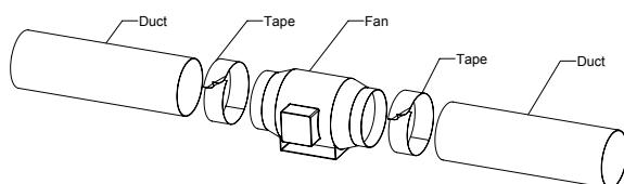
*To ensure quiet operation of ENERGY STAR qualified inline and remote fans, each fan shall be installed using sound attenuation techniques appropriate for the installation. For bathroom and general ventilation applications, at least 8 feet of insulated flexible duct shall be installed between the exhaust or supply grille(s) and the fan. For remote ventilation applications, where metal duct is generally required by code, a metal sound attenuator shall be installed between the hood and the fan.*
