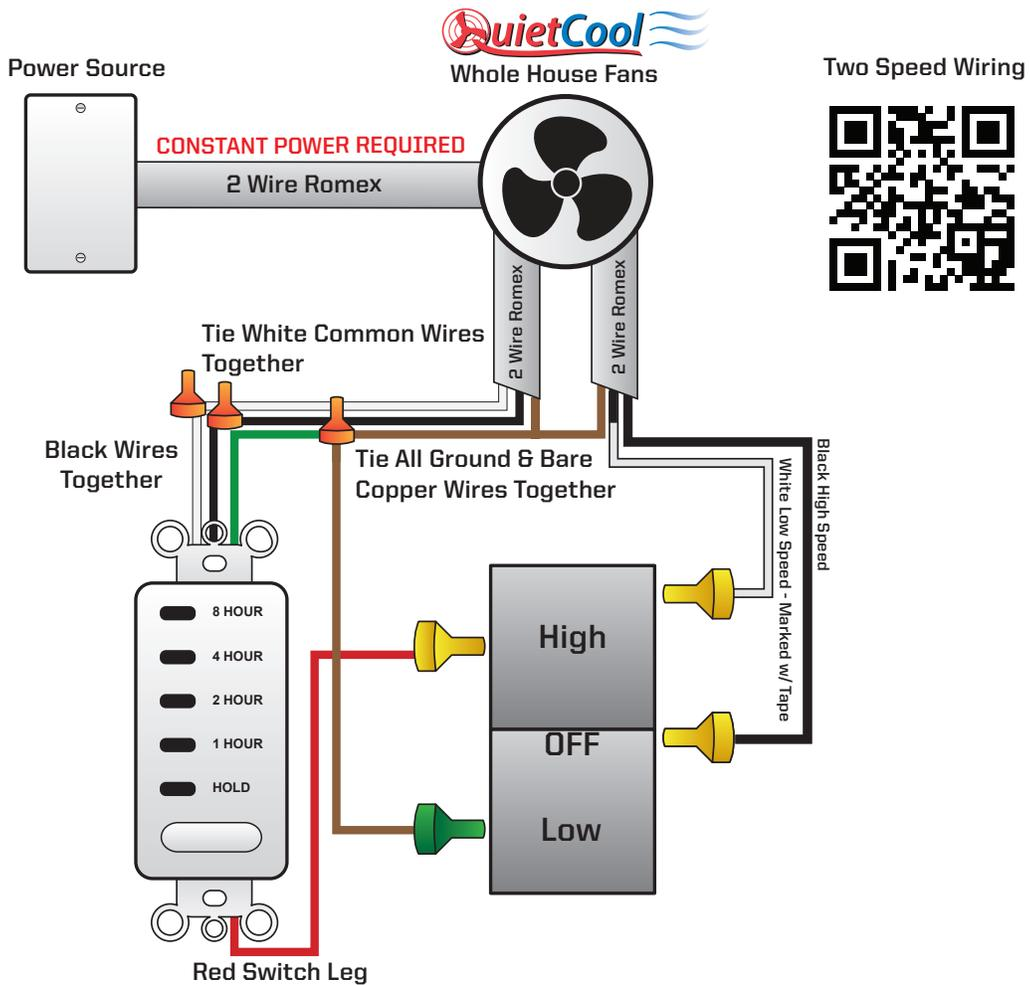
8. Feed the 2 wire Romex from your timer into the handy box. Feed the 2 wire Romex from your power source into the handy box.
