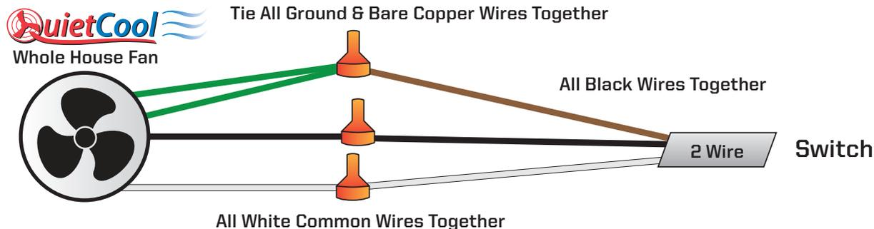
5. Begin wiring the fan by opening up the handy box. Take off the wire nuts within the handy box.
