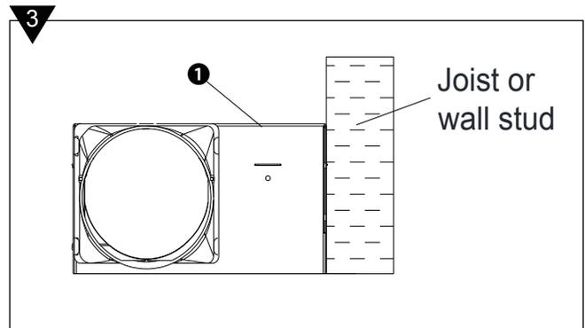
4. Mount the Fan Body **1** to the joist or stud using nails (not included) where indicated.
