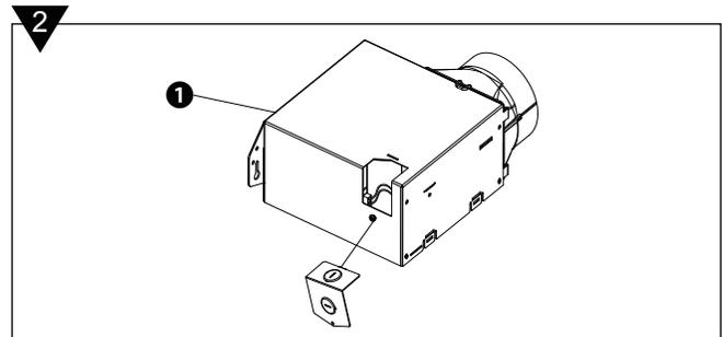
3. Place the Fan Body **1** next to a ceiling joist or wall stud. The Fan Body **1** should be level and perpendicular to the joist or stud.
