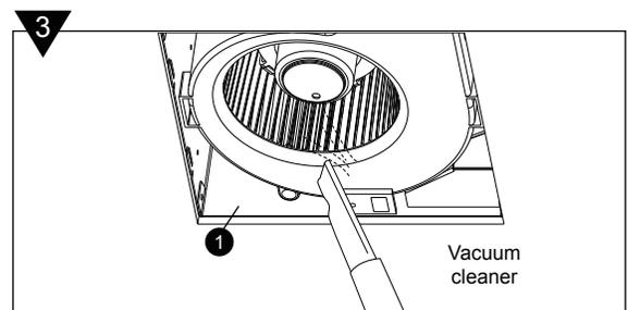
4. Dampen cloth with dust detergent and wipe the fan body **1** . Then wipe dry with a clean cloth.
