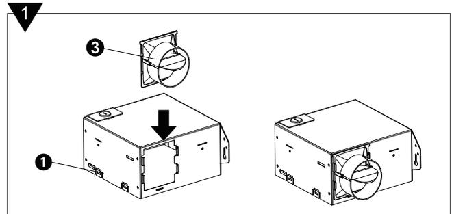
2. Remove the wiring box cover from the Fan Body **1**. Remove the wiring knockout from the wiring box cover with a flathead screwdriver (not included).
