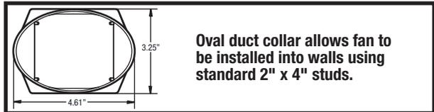
Oval duct collar allows fan to be installed into walls using standard 2" x 4" studs.
