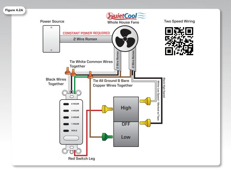
8. Feed the 2 wire Romex from your timer into the handy box. Feed the 2 wire Romex from your power source into the handy box.
