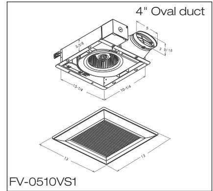
120V/60Hz. Duct diameter shall be no less than 4". Optional 24 gauge steel, fire code rated 4" oval to 3" round duct adaptor sold separately (Model # FV-VS43R). Fan can be used to comply with ASHRAE 62.2, LEED, EarthCraft, California Title-24 and WA Ventilation Code.
