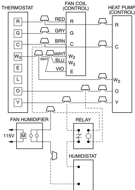
Fig. 20 – Wiring Layout of Humidifier to Heat Pump
