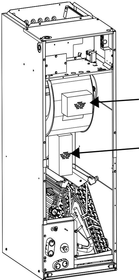
Fig. 1 – Remove Shipping Blocks
