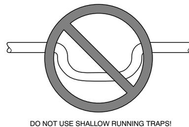
Fig. 18 – Insufficient Condensate Trap
